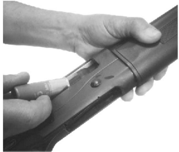
**Figure 10. Place shell into breach**
