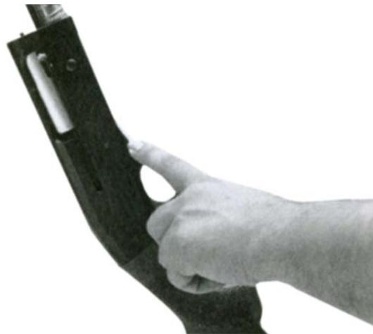
**Figure 13. Magazine shell latch**
