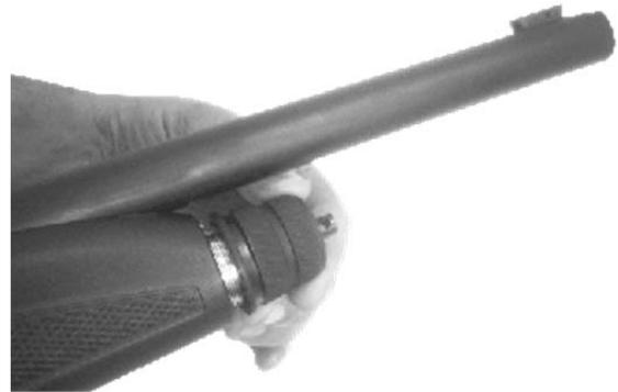
**Figure 8. Screw cap onto threaded magazine**
