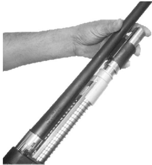
**Figure 6. Assemble barrel while centering magazine and receiver**
