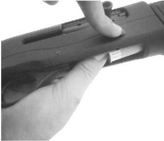
**Figure 9. Draw bolt into open position**
